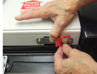
E. Make sure the metal memory card cover is sealed. If not, seal with a new seal from Ziploc bag of supplies.
