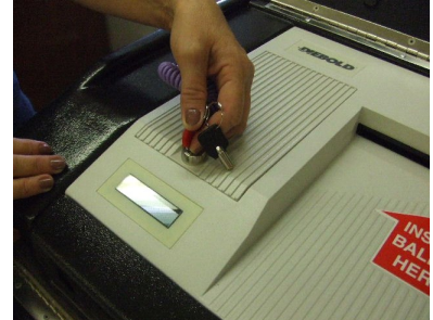
F. Using the red key, open and remove the printer cover and set it aside.
