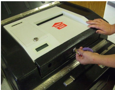
D. Using the brass key, unlock and open the front access gate located in front of the Optical Scan Tabulator.
