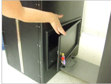
B. One judge must unlock and open all auxiliary compartments with the brass key on the Supervisor Card key ring to make sure they are empty.
