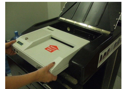
I. Slide the Optical Scan Tabulator back into place by making sure the unit is snug against the back of the ballot box.
